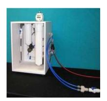
The system can be bench or shelf-mounted up to 8 feet away from the hydrogen generator. For the user's convenience, the included purity monitor can be located up to 6 feet away from the system.
